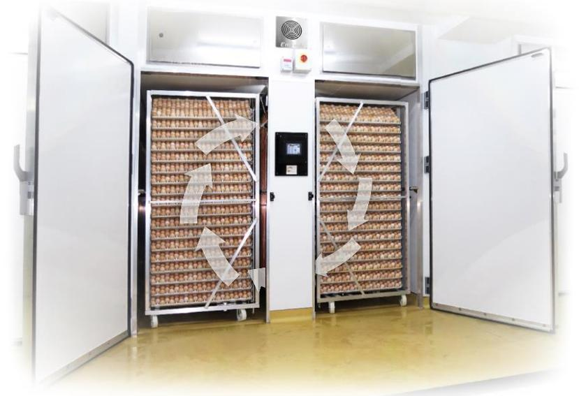
Perfect **air-flow** with only **one trolley** positioned each side of the **bi-directional fan**
