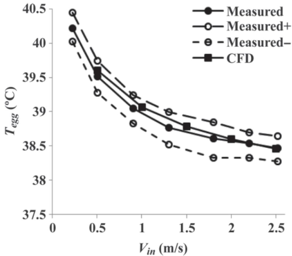
**Figure 3.** The average eggshell temperature,  $T_{egg}$ , versus inlet air velocity,  $V_{in}$ , for horizontal flow with an ambient temperature ( $T_{amb}$ ) = 37.36°C and a heat production of the egg ( $Q_{egg}$ ) = 285.6 mW, as simulated with computational fluid dynamics (CFD) and measured by Van Brecht et al. (2005). Measured = average value; Measured± = average value ± accuracy of the thermocouple ± SD of measured values.
