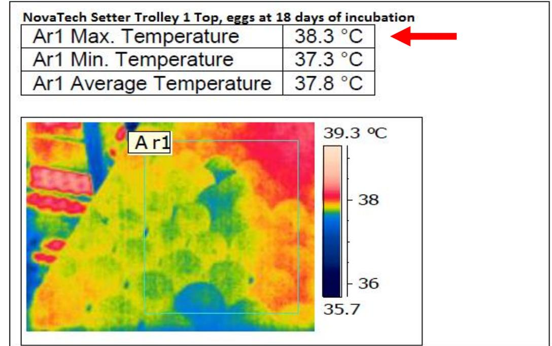
Thermal Image of a tray of eggs showing the egg shell temperatures with embryos at 18 days of incubation from the new NovaTech Setter, same trolley and position – Trolley 1 – Top. Note that the temperatures are within the ideal range of between 37.8°C and 38.3°C. The blue colour would be indicative of infertile eggs
