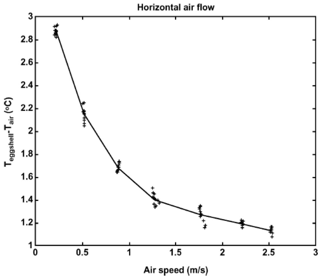
FIGURE 6. The temperature difference between the air and the eggshell as a function of the air speed of a horizontal airflow at 285.6 mW of sensible heat production.
