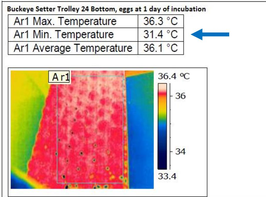
Thermal image from a Buckeye Setter, trolley 24 bottom, looking at eggs freshly set and only 1 day into incubation, shows a minimum temperature of only 31.4°C and has an average temperature of 36.1°C with a maximum temperature of only 36.3°
