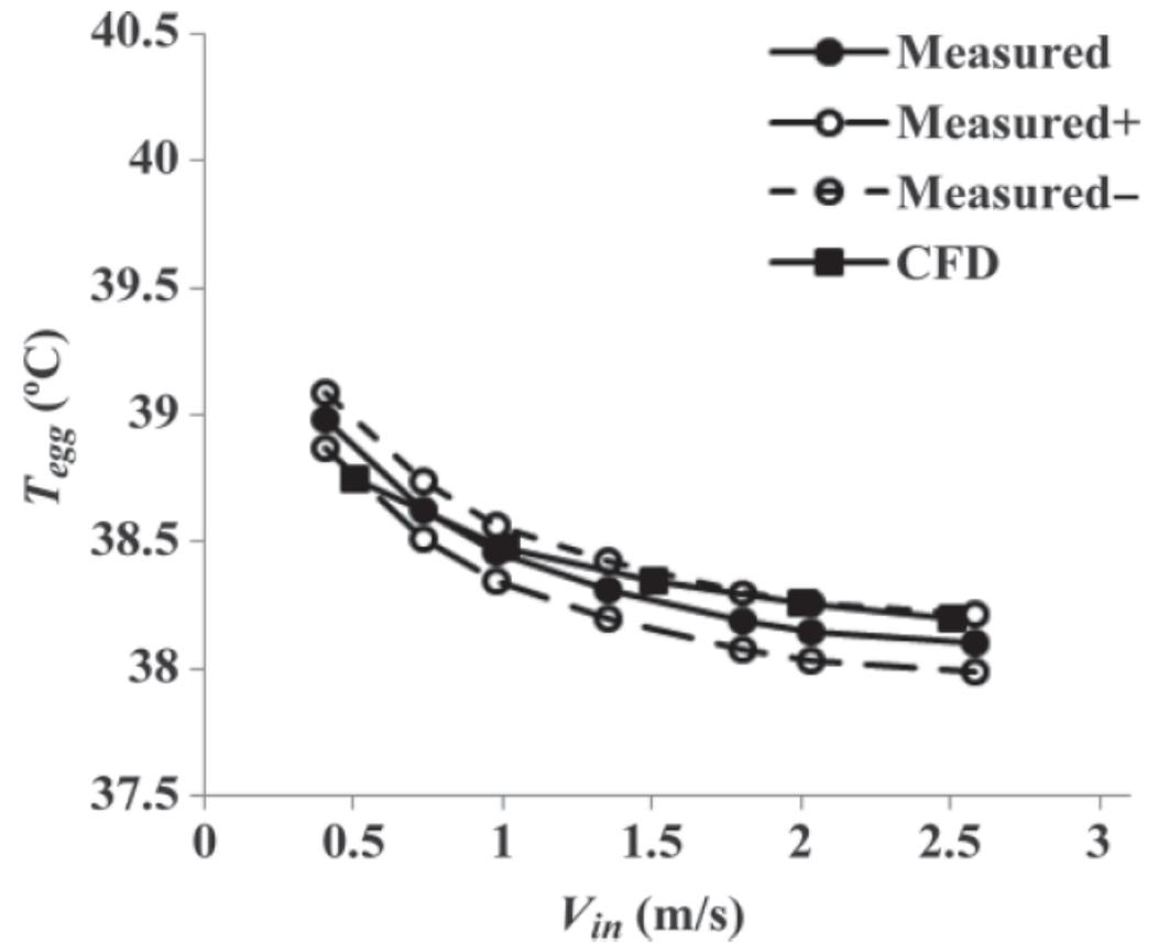
**Figure 10.** The average eggshell temperature,  $T_{egg}$ , versus inlet air velocity,  $V_{in}$ , for vertical flow with an ambient temperature ( $T_{amb}$ ) = 37.80°C and a heat production of the egg ( $Q_{egg}$ ) = 150.7 mW, as simulated with computational fluid dynamics (CFD) and measured by Van Brecht (2004). Measured = average value; Measured± = average value ± accuracy of the thermocouple ± SD of measured values.
