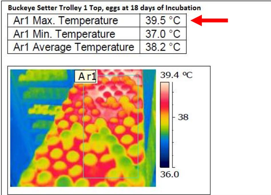
Thermal Image of a tray of eggs showing the egg shell temperatures with embryos at 18 days of incubation from a 10 year old Buckeye Setter, from the top of Trolley 1 (first trolley from the front on the left). Note temperatures in excess of 39.4°C, which can be detrimental to chick quality. The lighter yellow and green are likely to be indicative of infertile eggs.
