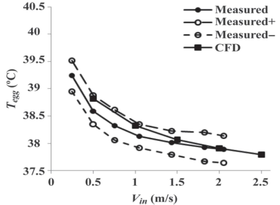
**Figure 4.** The average eggshell temperature,  $T_{egg}$ , versus inlet air velocity,  $V_{in}$ , for vertical flow with an ambient temperature ( $T_{amb}$ ) = 37.06°C and a heat production of the egg ( $Q_{egg}$ ) = 288.7 mW, as simulated with computational fluid dynamics (CFD) and measured by Van Brecht et al. (2005). Measured = average value; Measured± = average value ± accuracy of the thermocouple ± SD of measured values.
