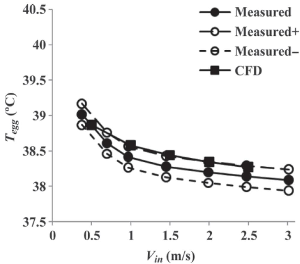
**Figure 9.** The average eggshell temperature,  $T_{egg}$ , versus inlet air velocity,  $V_{in}$ , for horizontal flow with an ambient temperature ( $T_{amb}$ ) = 37.70°C and a heat production of the egg ( $Q_{egg}$ ) = 148.5 mW, as simulated with computational fluid dynamics (CFD) and measured by Van Brecht (2004). Measured = average value; Measured± = average value ± accuracy of the thermocouple ± SD of measured values.
