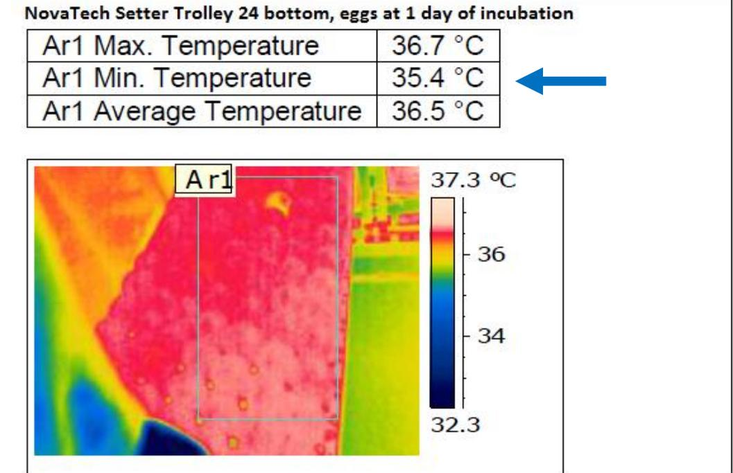
Thermal image from the NovaTech Setter trolley 24 bottom, note the much higher temperatures, showing a minimum temperature of 35.2°C, an average temperature of 36.5°C and a maximum temperature of 36.7°2
